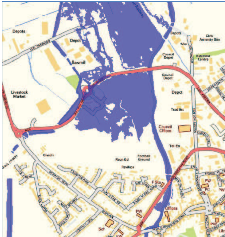
Figure 13 - Sensitivity to flow: November 2012 hydrology; blockage 95%; 80% scaling to JBA 35.9 m 3 /s
