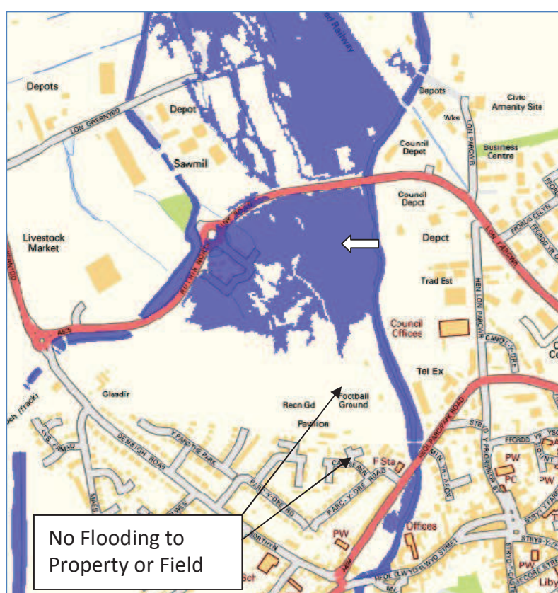
Figure 12 - Sensitivity to flow: November 2012 hydrology; blockage 95%; 70% scaling to JBA 31.4 \text{ m}^3/\text{s}
