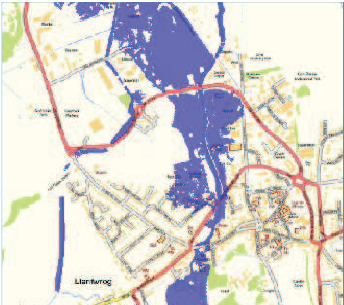
Figure 34 - Option 5- ISIS TUFLOW Model Results for 1 in 100 year return period with Climate Change and 95% blockage
