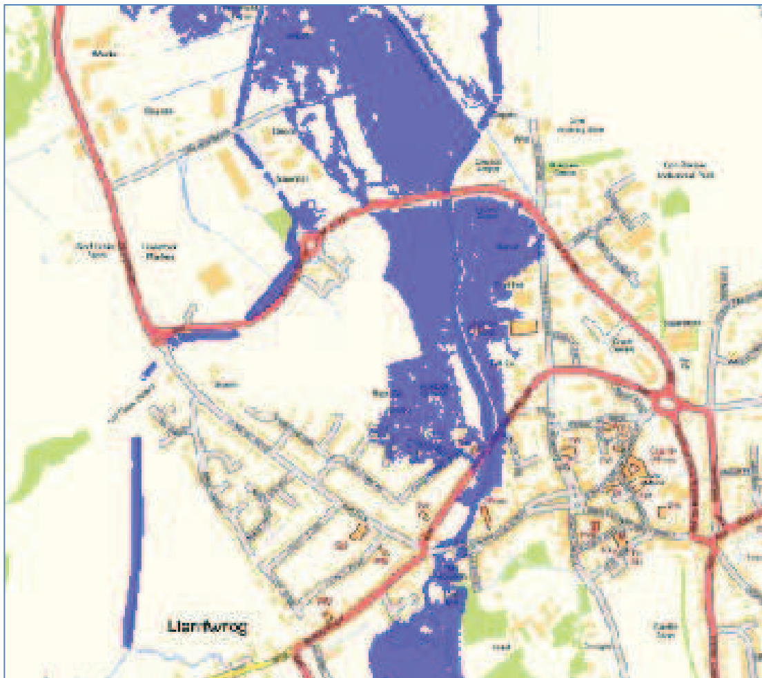
Figure 25 – Option 2 - ISIS TUFLOW Model Results for 1 in 100 year return period with Climate Change and 95% blockage
