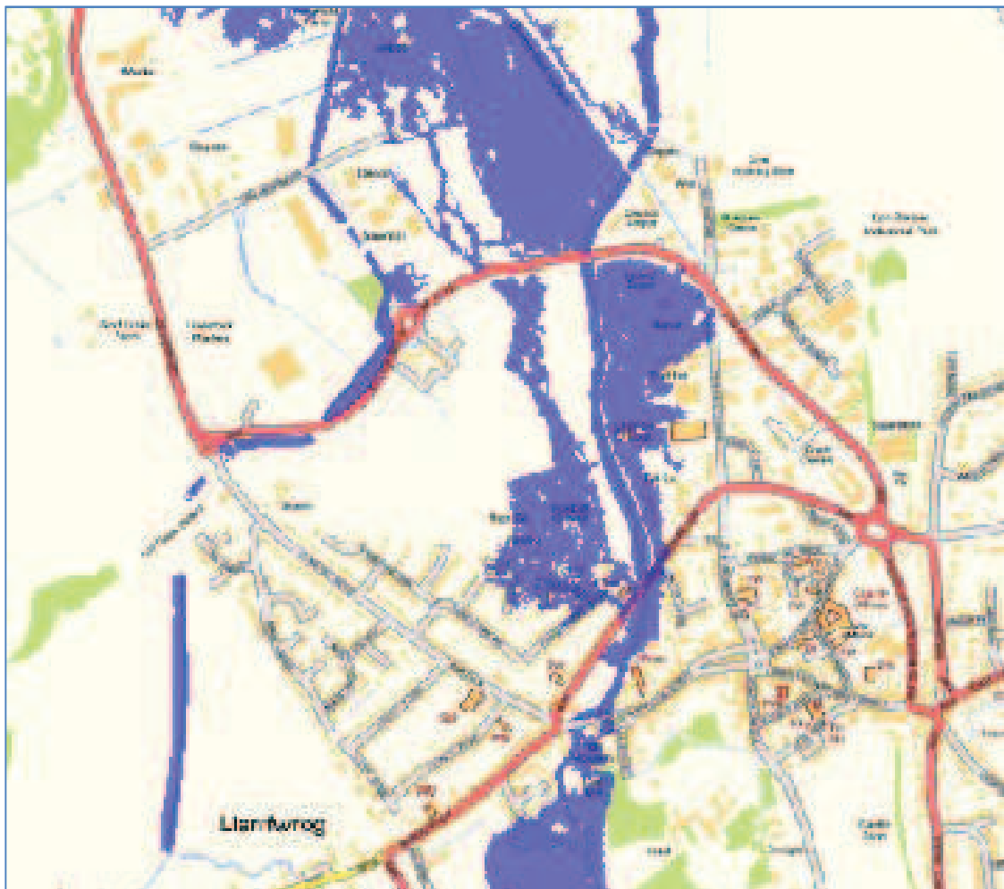
Figure 28 - Option 3 - ISIS TUFLOW Model Results for 1 in 100 year return period with Climate Change and 95% blockage
