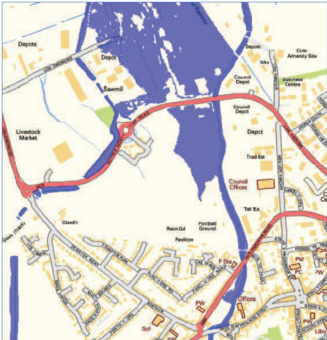
Figure 6 - Design hydrology; Q = 1 in 100 years, 35.2 m 3 /s Blockage = 0%: (Scenario B)
