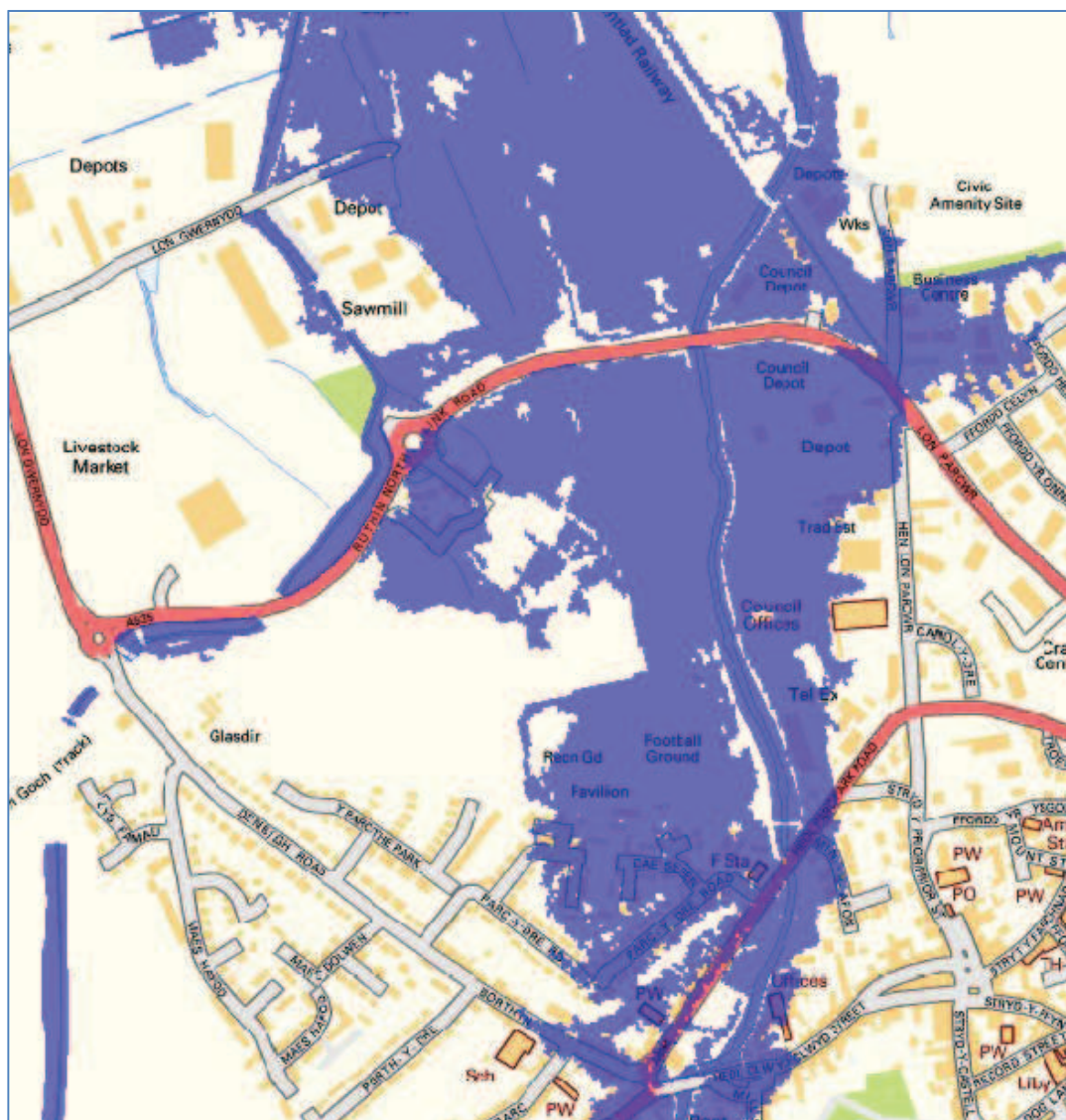
Figure 8 - Design hydrology; Q = 1 in 1000 years, 59.2 m 3 /s: Blockage = 0% (Scenario B)
