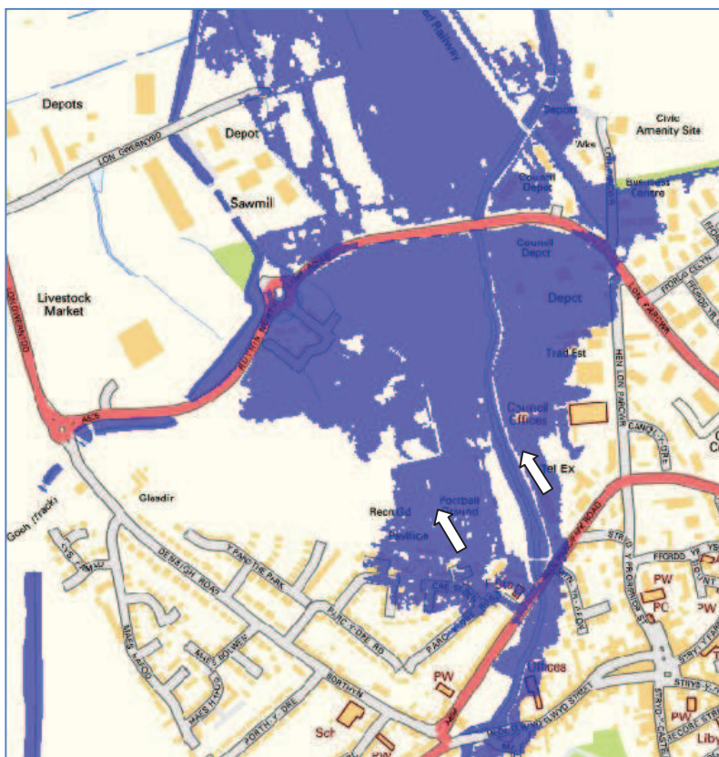
Figure 14 - Sensitivity to Flow: November 2012 hydrology; blockage 95%; 100% scaling to JBA 44.9 m 3 /s
