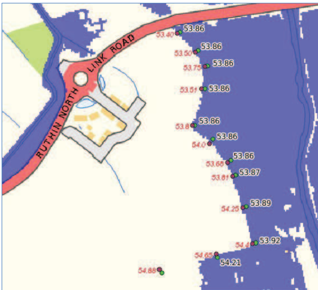
Figure 24 - Comparison of modelled peak water level for the 1 in 100 yr return period with Climate Change and 95% blockage, and existing embankment level. Existing embankment levels shown in red; modelled levels shown in black.
