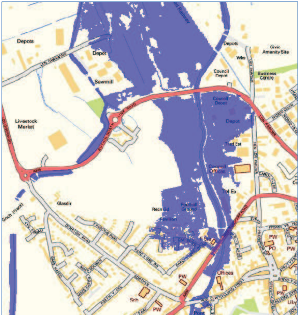
Figure 7 - Design Hydrology; Q = 1 in 100 years plus Climate Change, 42.1m 3 /s Blockage = 0% (Scenario B)
